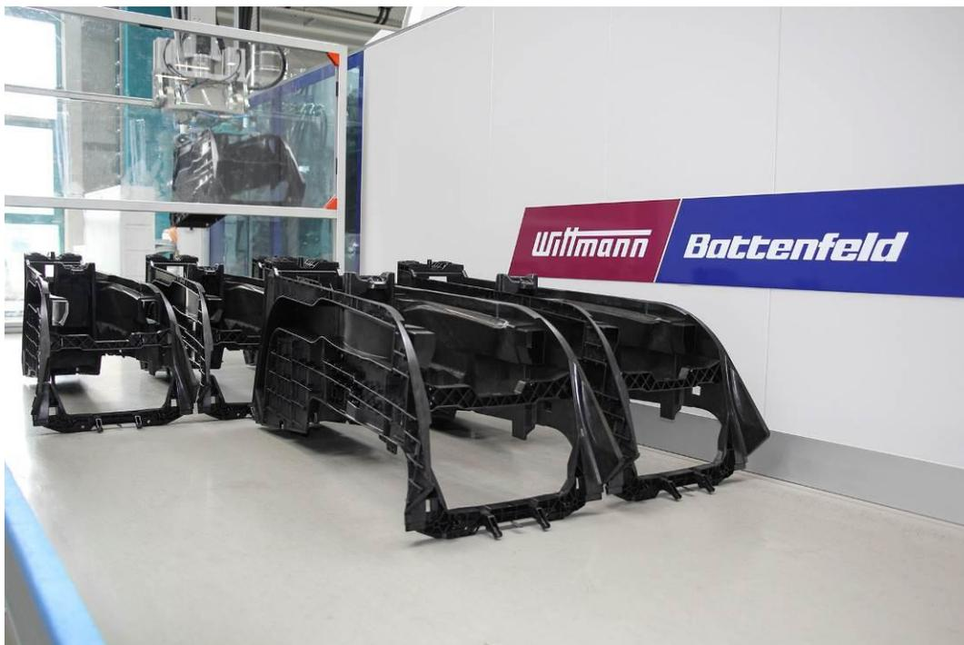
**Fig. 6:** Support for a passenger car center console (Photo: WITTMANN BATTENFELD)
